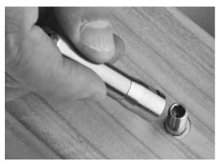
Make sure the post side of the Push-Lock<sup>TM</sup> Lag is flush against the post.
